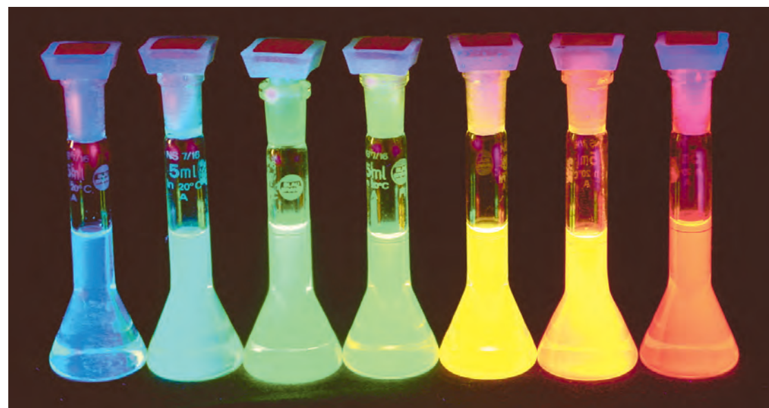
Fluorescent light changes depending on the size of CdSe-based quantum dots
